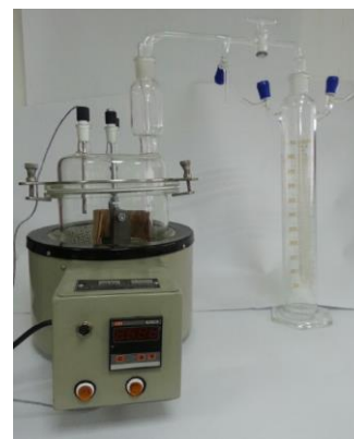
Fig.2 Power transformer oil measurement setup.
