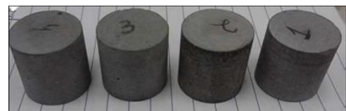
Fig. 2 Cement plugs employed for lab testing of strength
