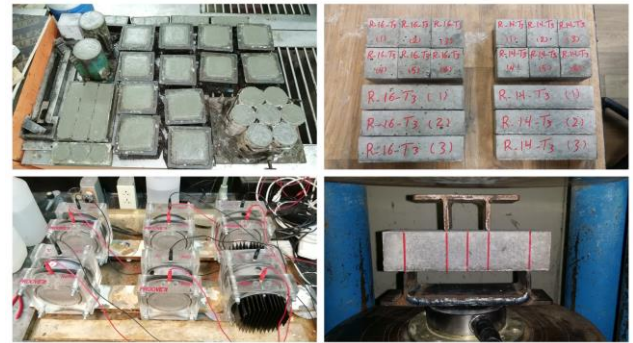
Fig: Treated Crumb Rubber Concrete Samples
